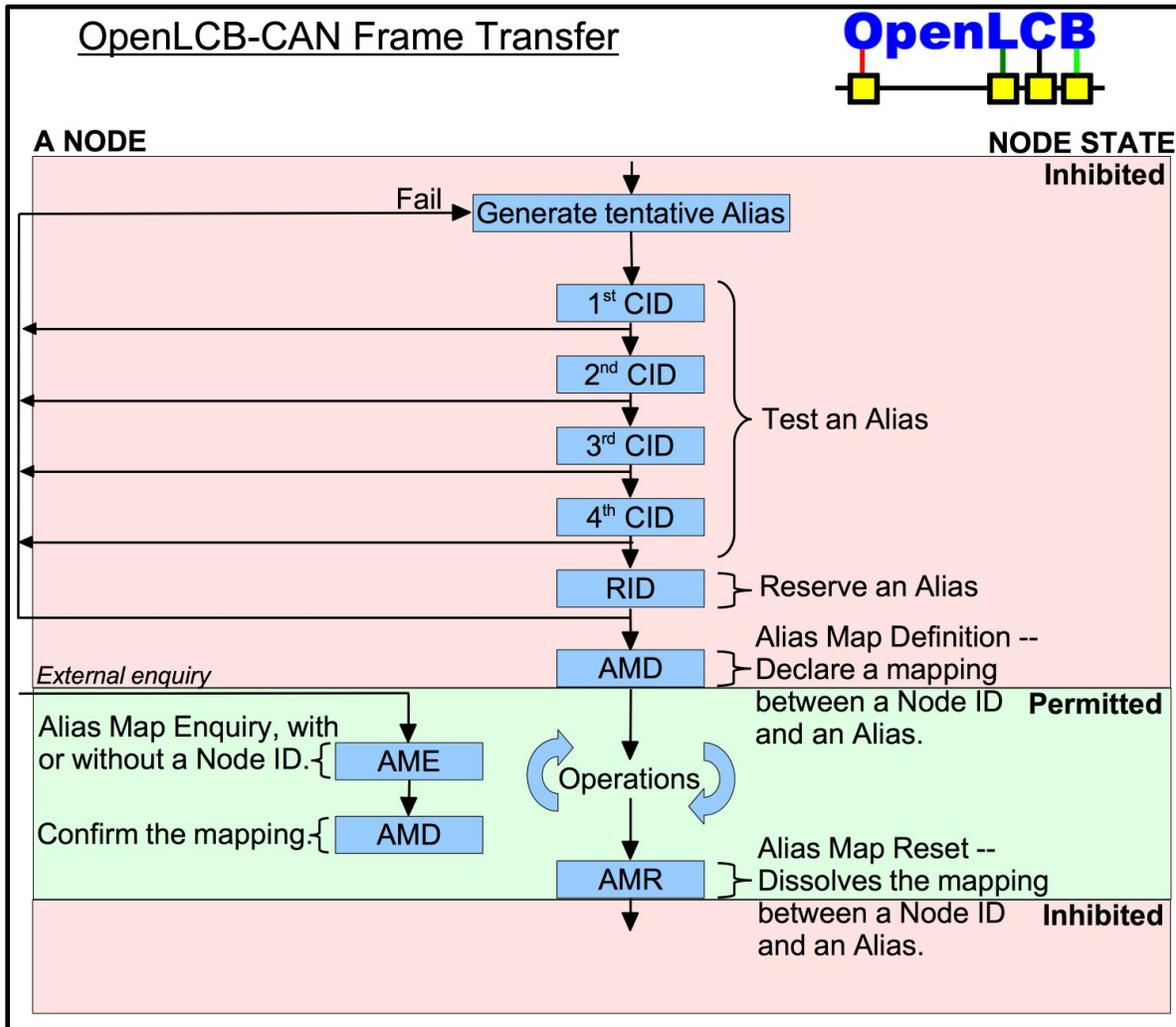
365 Note that in the diagram above, the 'Fails' are due to the node receiving a message which uses its tentative Alias, and it therefore needs to back off and try a new tentative Alias.
