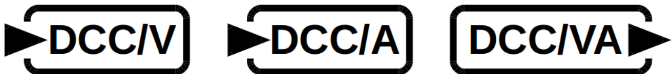
Figure 3: Example graphics depicting, from left to right, a DCC Voltage Mode Consumer, DCC Current Mode Consumer, DCC Voltage & Current Mode Source. Other variations are also possible.
